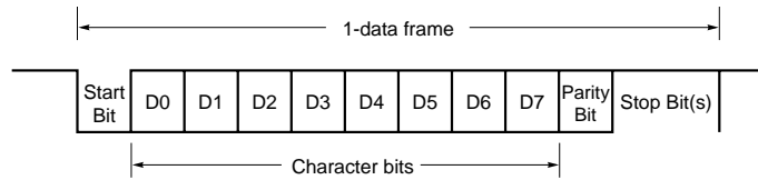
Figure 16-7. Asynchronous Serial Interface Transmit/Receive Data Format
